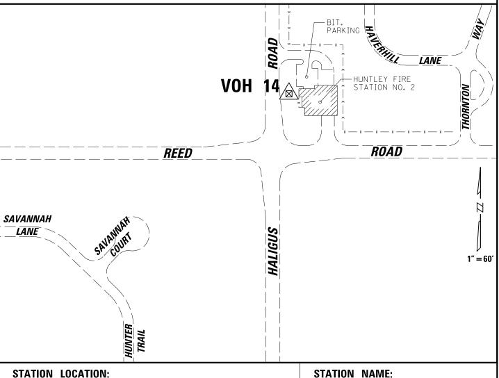
2" BRONZE DISC SET IN CONC. SIDEWALK ON SOUTH SIDE OF WEST DOOR OF HUNTLEY FIRE STATION NO. 2.
